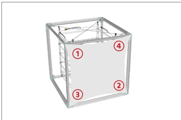
**Step 9:** Fold silicone edge graphics over an install into first corner of frame working outwards 4-6 inches. Repeat on remaining corners starting with the opposite corner. Follow the Graphic Diagram.
