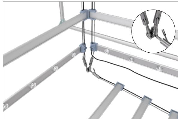
**Step 8:** Attach power cables between bottom and 1 vertical light array. Not all LED Light Arrays need to be plugged in at bottom. 3 plugs will hang freely.
