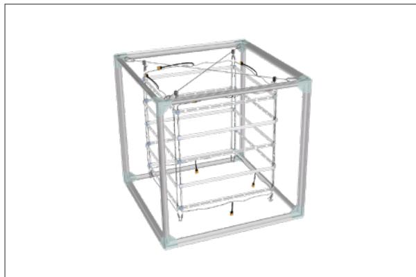
**Step 7:** Attach bottom horizontal LED Light Array to 4 corners of vertical LED Light Arrays.
